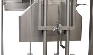
The height and the distance to the products can easily be adjusted to compensate for different bird sizes.
