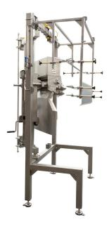
The frame is designed to hinge the module in-line or off-line to allow for proper cleaning and to ease maintenance. The motor is automatically switched off when the frame is opened as a safety measure.
