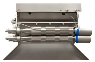
The pulling mechanism consists of two stainless steel rollers, placed above each other and rotating in opposite direction. The tail feathers are guided into the machine, between the rotating rollers. The rollers are provided with a profile, which pulls the tail feathers between the two rollers and out off the feather follicle. A guide above the rollers protects the thighs of the birds from being damaged. The machine is provided with a water spray system for draining dirt and feathers.
