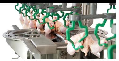
The breast cap cutter gives an exactly positioned, constant and symmetrical cut. This allows for a maximum of valuable breast meat to be left with the cap while minimizing bone contamination of untrimmed filets in the form of ribs. The module can cut the ribs at variable lengths. The module is placed after the HY wing cutter.
