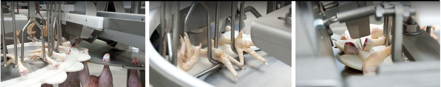
**The Meyn Syncom rehanger slaughtering-evisceration assures a smooth transfer of the products from the slaughtering line to the evisceration line. Both line speeds and positions are accurately synchronized for optimum performance.**
